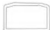
Rectangular shape allows for laser detectors to be mounted directly to the rod – no bracket required!
